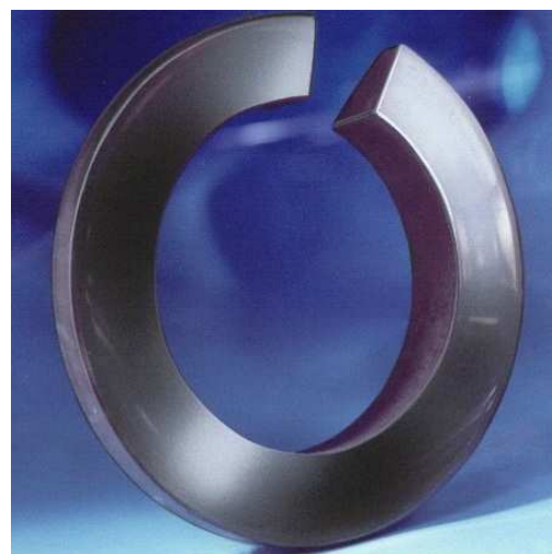
Fig. 10: Running surface of a carbon sealing ring after 10.000 hours of operation
